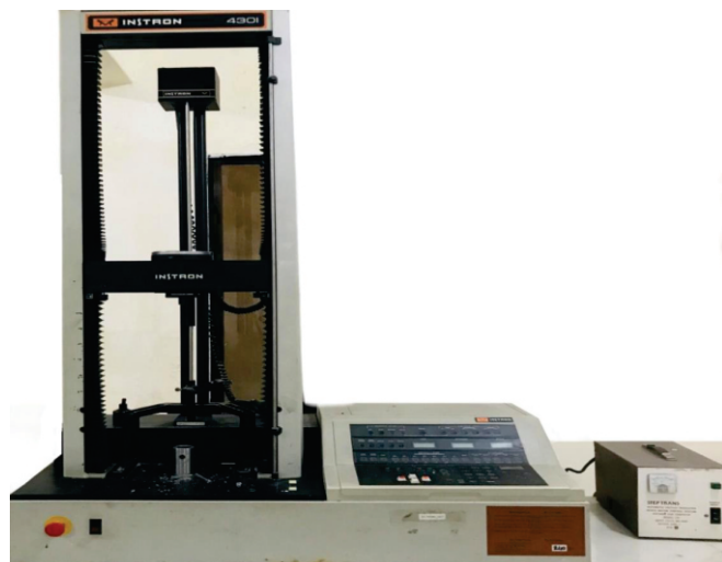
Figure 2: Instron 4301 Universal Testing Machine (Used for Tensile, Compression, Shear, Fatigue, Friction, and Flex Tests)
