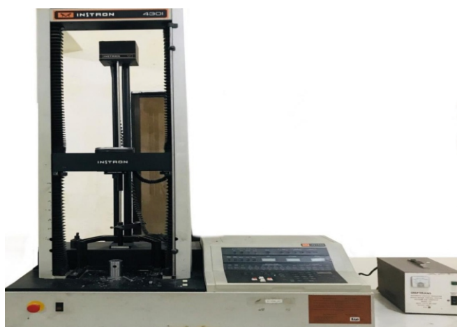
Figure 2: Instron 4301 Universal Testing Machine (Used for Tensile, Compression, Shear, Fatigue, Friction, and Flex Tests)
